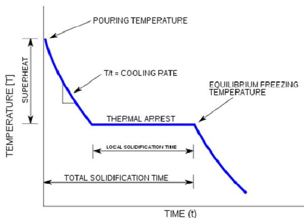
Fig. 1. The cooling curve
