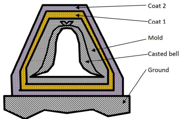
Fig. 4. The complete coating of the cooling mold
