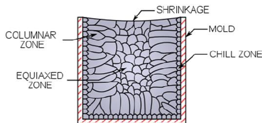
Fig. 2. The grain macrostructure
