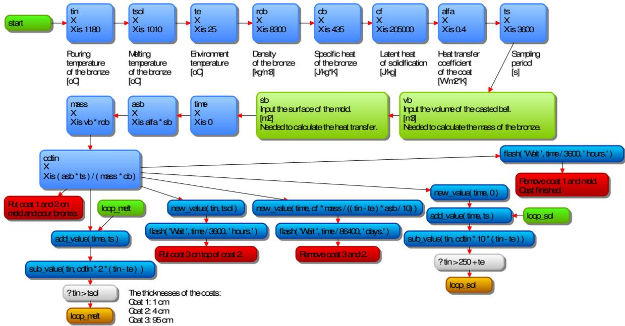
Fig. 5. The VisiRule implementation of the control algorithm
